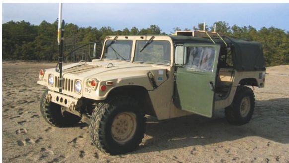
The US military has mounted prototypes of the Anywave GSM base station on Humvees.
