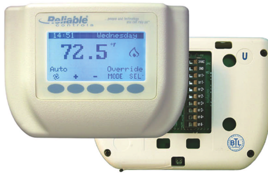
Figure 2 The Mach-Vision, a programmable user interface from Reliable Controls, communicates using the BACnet (Building Automation and Control Network) Protocol.
