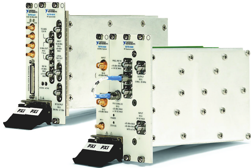
These National Instruments RF modules are representative of CompactPCI-based PXI's modular architecture. The modules require a card cage that includes power supplies and cooling facilities. Each cage must also include a slot-zero module. Many slot-zero modules are full-featured embedded PCs.
